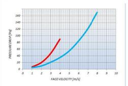
Pressure Drop vs Air Inlet Air Flow: Pressure Drop through the InoVane® Water is low due to its airofoil design. Pressure Drop is based upon laminar air flow in the units, other pressure drops caused by shape of aggregates, frames aso is not taken into consideration. This is valid for the system water / Air @ 20°C and 1 bar. Data achieved with uniform load and flow.
