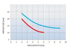
Drop Size limit vs Face Velocity: The InoVane® Water separator has a droplet removal efficiency of 100% for water droplets 12-15 microns and larger. The limitation to drop size means the smallest drop which is completely separated by the system. The limit drop size is measured in microns (0,001 mm = 1/1000 mm). As example a normal human hair is 75-200 µm. Rain drop appr. 200-10,000 µm. Mist appr. 80 - 200 µm.
