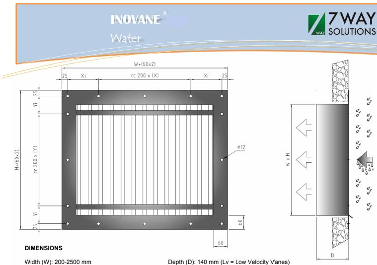
Width (W): 200-2500 mm Height (H): 200-2500 mm Distance: X & Y (To be calculated) Depth (D): 140 mm (Lv = Low Velocity Vanes) Depth (D): 210 mm (Hv = High Velocity Vanes) Distance: Xi & Yi (Max 200 mm)
