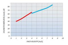
Sound Power Levels vs Air Inlet Air Flow: Sound Power Levels is based upon laminar air flow in the units, added noise caused by shape of aggregates, frames a.s.o is not taken into consideration.
