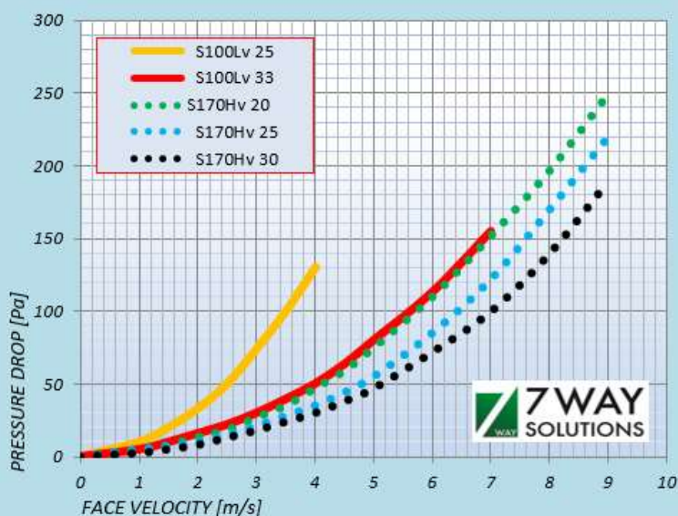
Single / 1:st Stage; InoVane® Vane Droplet Separator
