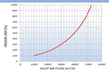
Pressure Drop vs Air Inlet Air Flow:
