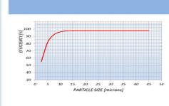
Efficiency vs Particle size: The InoVane Tempest has a dust removal efficiency of 98% for particles 15 microns and larger. This graph provides complete data on particle size removal efficiency showing that it will remove over 93% of all solid particles 8 micron or larger. In addition the InoVane Tempest has a water removal efficiency of over 90%.
